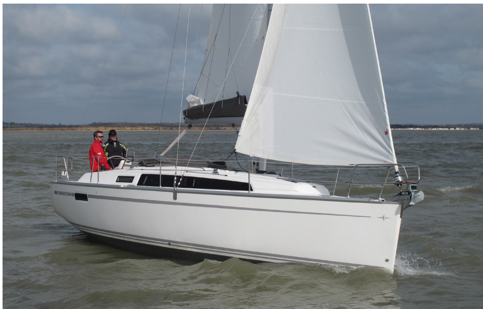
A light modern cruiser makes more leeway when hove to than her traditional counterpart
